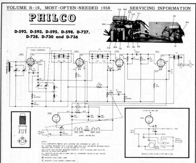
Above is an exact circuit for Models D-592, D-593, and D-595. For differences in Models D-727, D-728, D-730, and D-736, refer to clock circuit in insert above. Model D-598 uses a neon lamp as an off-on indicator, and incorporates a phonoinput jack, a variable tone control, and a radio-phono switch.
