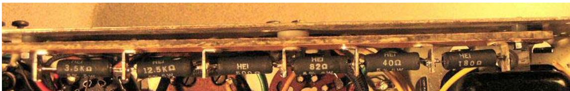
This angle clearly show the chassis standoffs on the mounting screws at each end as well as the glued on standoff in the middle to absolutely prevent shorting of the screw heads from flexing against the chassis.
