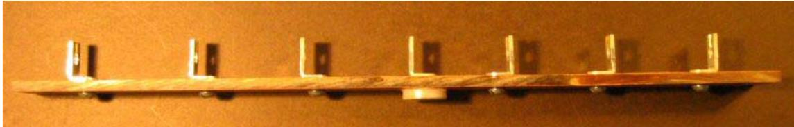
The L threaded brackets were then laid out to get the spacing needed for the number of resistors to be used, taking into account the size of the resistors. The L brackets were secured to the phenolic board with 4-40 screws into the threaded portion of the mounting brackets. One source is Digi-key <http://dkc3.digikey.com/PDF/T053/1454.pdf>
